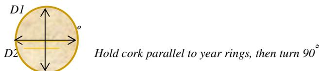
Diameter 1(D1) – Diameter measured on the cork growth rings.
